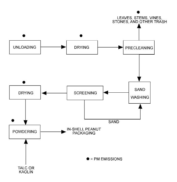
Figure 2-1. Typical in-shell peanut processing flow diagram.
