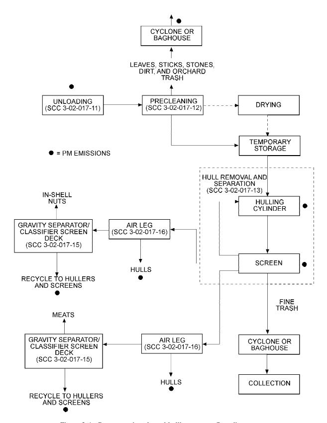
Figure 2-4. Representative almond hulling process flow diagram.
