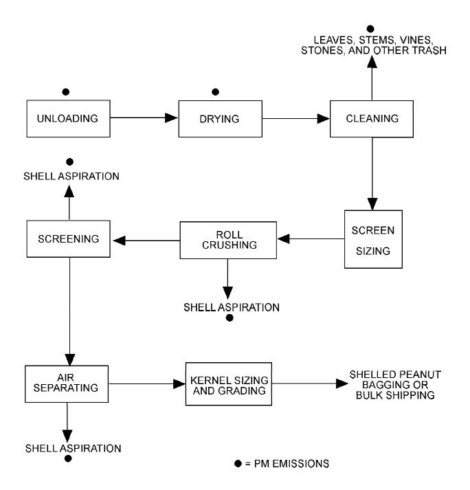
Figure 2-2. Typical shelled peanut processing flow diagram.
