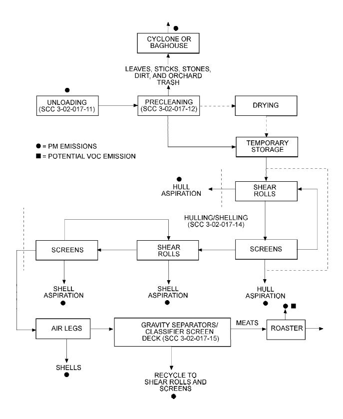
Figure 2-5. Representative almond huller/sheller process flow diagram.
