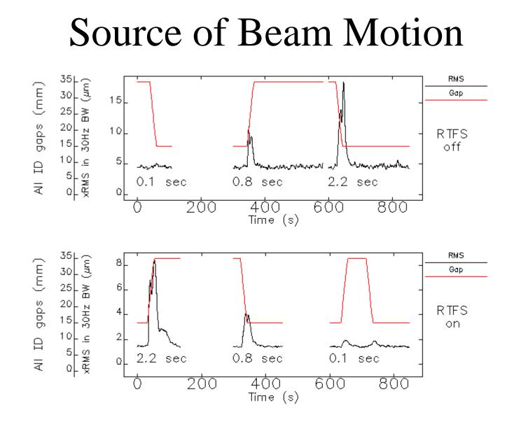
Reduction of RMS motion with reduction of DC OC interval.
