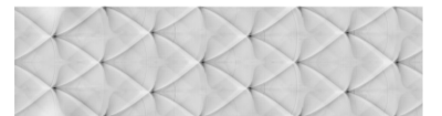
The time history of the released chemical energy shows the detonation cells.
