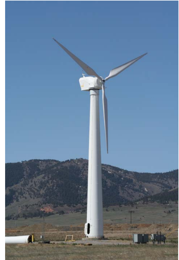
NW100B 100-kW wind turbine
