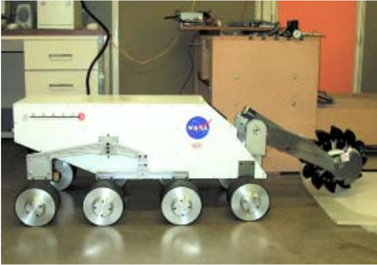
At 0.91 meters (3 feet) long, this prototype excavator is the same size as the finished product intended to be sent to the Moon to purify lunar soil for use as propellant. According to Michael Duke, director of the Center for Commercial Applications of Combustion at the Colorado School of Mines in Golden, the wheel on the end of the boom can dig up several times the weight of the device — 45.36 kilograms (100 pounds) — in dirt each hour.
