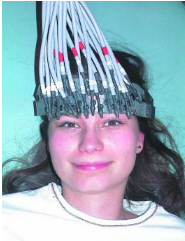
Optical fibers carrying near-infrared laser light dangle from the diffuse optical tomography (DOT) imaging device worn by this volunteer. Researchers can measure blood activity and deduce brain functions by measuring the scatter and absorption of light shining on the brain.
