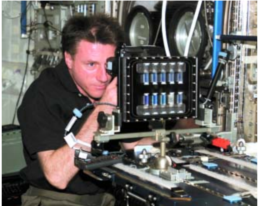
Expedition 8 Commander and Science Officer Michael Foale uses a digital still camera to photograph a Slow Growth sample module for the Binary Colloidal Alloy Test (BCAT)-3. In BCAT-3, Principal Investigator David Weitz of Harvard University, Cambridge, Massachusetts, is studying the long-term behavior of three classes of colloids to better understand their assembly and thermodynamics and how to engineer their properties.
