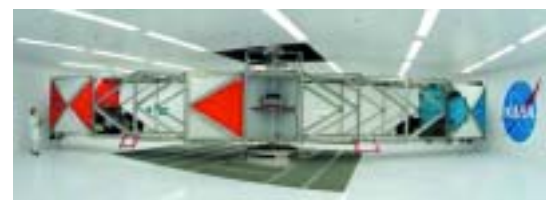
A long-arm centrifuge exposes the body to a continuous amount of artificial gravity. Scientists like William Paloski, Johnson Space Center, Houston, Texas, can use results of human experiments on long-arm centrifuges to design a rotating spacecraft. If all or part of a spacecraft were built to rotate, then astronauts in microgravity would be exposed to passive artificial gravity similar to the gravitational force humans are accustomed to on Earth.
