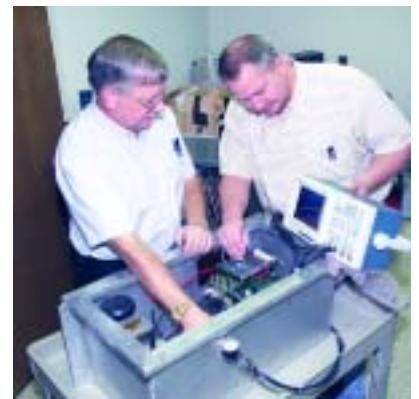
Dick Maurer (left) and Dave Roth (right) of the Johns Hopkins University Applied Physics Laboratory, Laurel, Maryland, check the response of neutron detector systems designed to measure previously unmonitored radiation that could be dangerous to astronauts. The detectors are mounted in the case that carried them approximately 26,000 meters (85,000 feet) into Earth's atmosphere during a balloon flight experiment, a test readying them for use in space.
