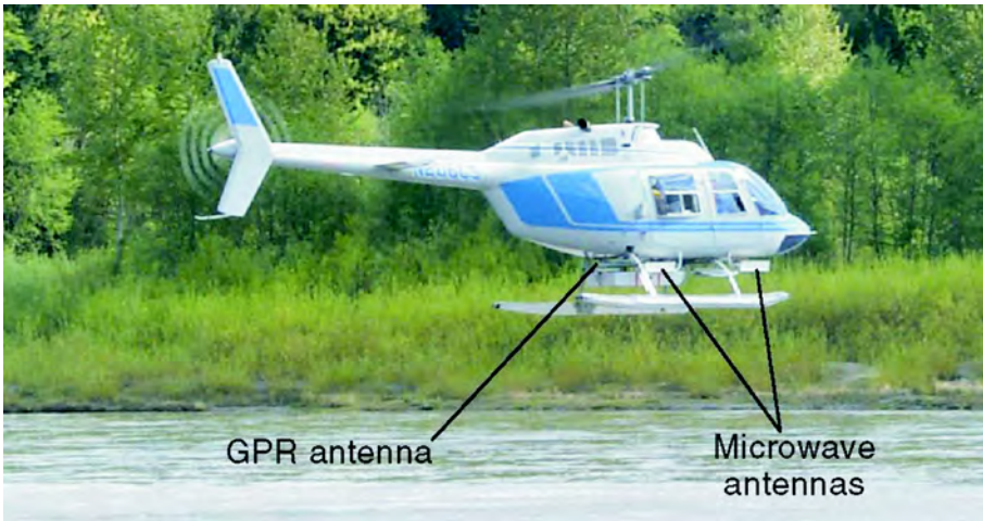
Figure 2. Helicopter-mounted radar experiment. Note the two microwave antennas located just below the cabin on both sides, and the GPR antenna located in the rear middle of the helicopter.
