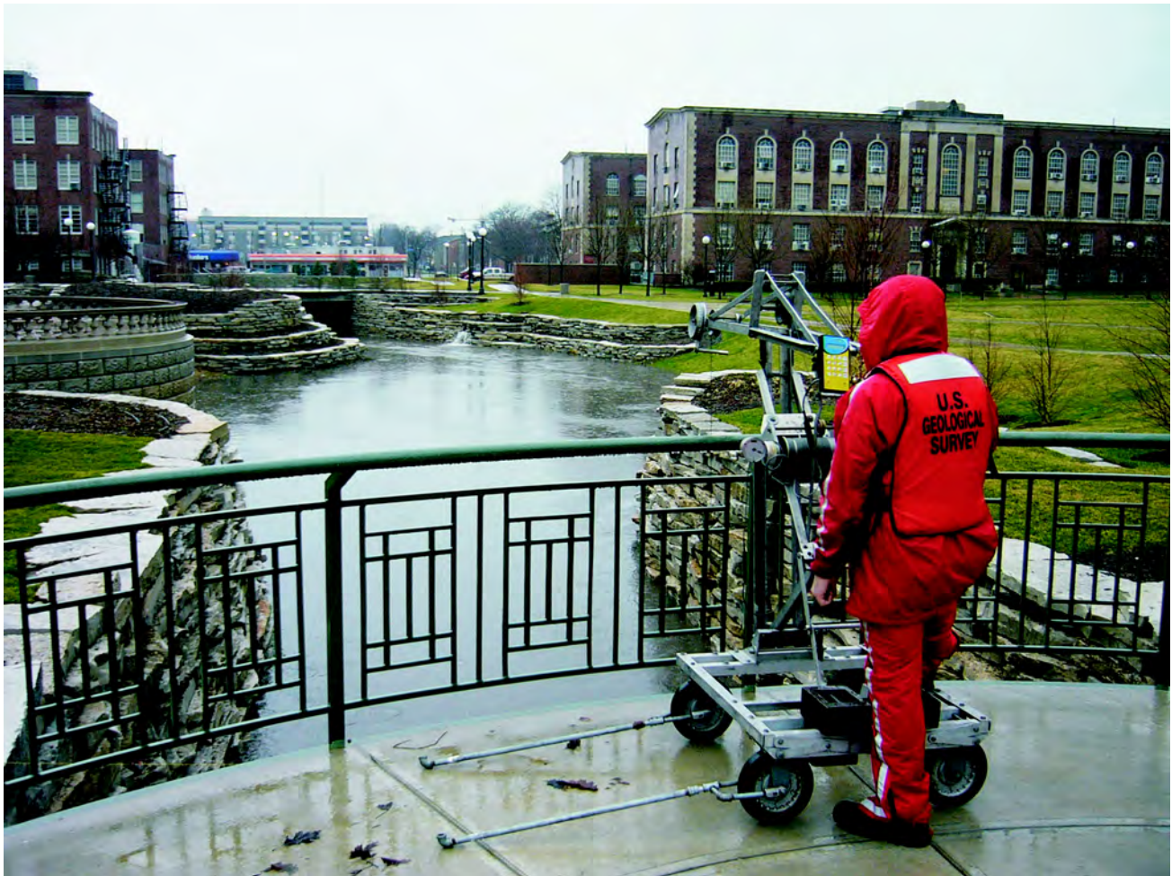
Figure 1. USGS Hydrologic Technician Phil Dennis making a conventional discharge measurement using a 4-wheel base, sounding weight, and spinning-cup current meter on the Boneyard Creek at Urbana, Illinois (University of Illinois Campus).
