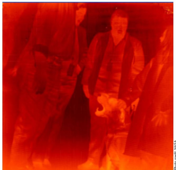
Caption Above: A false color image with the QWIP camera of engineers and a seeing-eye dog (named Denver). This image illustrates the slight difference in temperatures of the scene – dark red being coldest and orange the warmest. Note the hand visible inside the labcoat pocket and the very warm tongue of Denver, curled in a yawn. Also note the different hand temperatures of the people, some warm some cold.
