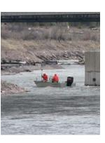
In this photo (left), US Geological Survey staff are shown navigating the Blackfoot River as they set up equipment to measure river velocities during spring flows. EPA is funding this work to evaluate pier scour and estimate the ability of fish to swim upstream (fish passage) on the Blackfoot River during
