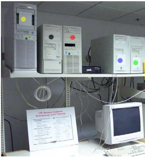
Fig. 5. The five-node active-network test bed we set up in our laboratory at NIST in order to conduct our experiments and to make measurements. The nodes from left to right: Yellow, Black, Red, Blue, and Green.
