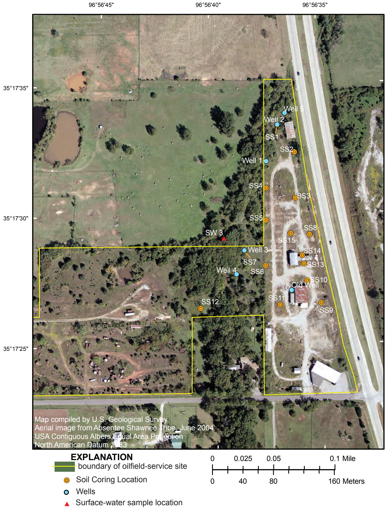
Figure 4. Locations of soil coring sites and installed wells (including existing supply well labeled Old Well) near Shawnee, Oklahoma, 2005–2006.
