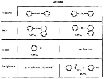
Conditions: 4 hrs at 250 C in FC-70 with 7 MPa H<sub>2</sub>.
