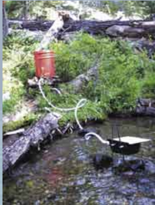
Example of an antimycin drip station used to remove non-native fish.
