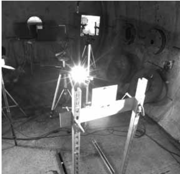
PRIOR TO TESTS of the Laser Area Defense System in the Explosive Components Facility, critical elements of the system were configured for stationary and spinning mortar targets.
