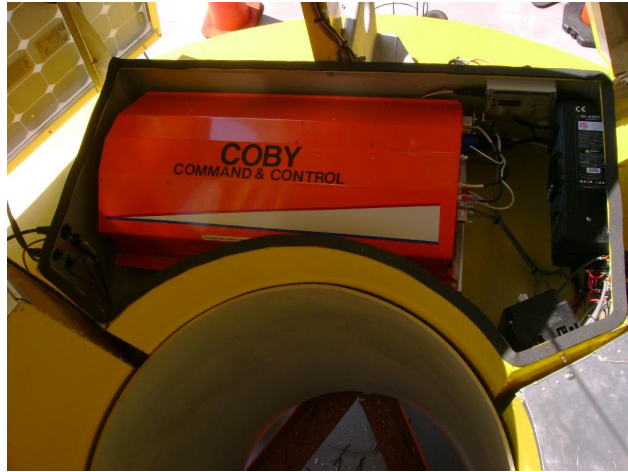
Figure 5. COBY Control Computer/Solar controller compartment on buoy deck without top cover.
