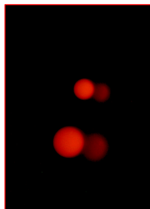
Fluorescence micrograph of pure rhodamine spheres produced by the IJPP. The sample is tilted to see the contact surface and the three-dimensional shape.
