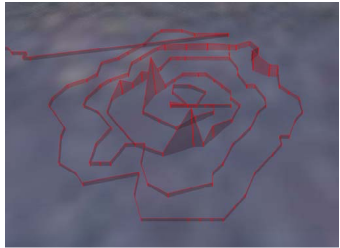
Fig. 13. A slanted view of the ocean area where the test was conducted. The measured rhodamine concentrations are shown as a vertical "ribbon" along the route taken by the OASIS boat (as shown in Figs. 11 and 12).
