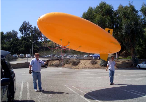
Fig. 7. The TAOSF aerostat observation platform. The aerostat is an unmanned, lighter-than-air (LTA) unpowered blimp on a tether. Helium is used for buoyancy.
