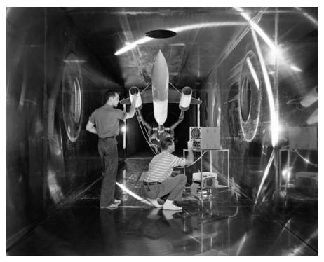
Engineers Check Body Revolution Model: 1957. (NASA)
