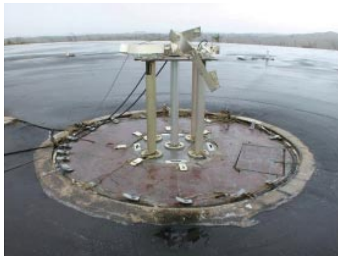
The remains of a VORTAC navigational aid stand testament to the power of Super Typhoon Pongsona.
