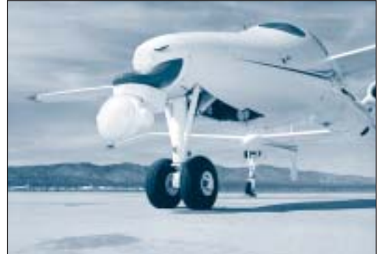
An AMphitech OASys Kaband radar was the primary sensor installed on Scaled Composites’ Proteus for the second phase of NASA-sponsored Unmanned Aerial Vehicle Detect, See and Avoid flight tests.
