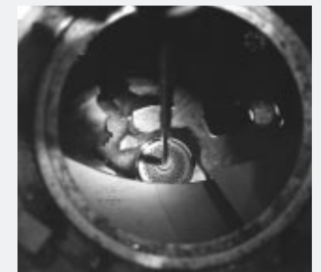
The last bit of extract containing the unstable germanium is drawn out from the gallium tank. The extract appears as a silvery pool floating on top of the duller, liquid gallium metal.
