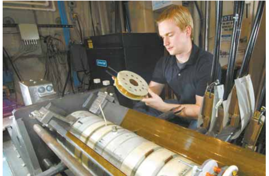
DEREK LAMPPA (5445) examines a coil that is part of a small-scale coil gun test bed. The test bed, in the foreground, includes four 50 mm coils used to test and refine electromagnetic acceleration of an aluminum projectile to as fast as 400 meters per second. (Photos by Randy Montoya)
