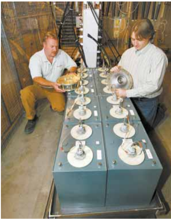
GARY FRANK and Matthew Aubuchon (both 5445) inspect a Sandia-developed capacitor bank that will become part of the full-scale coil gun system scheduled to be field tested at Sandia this summer.
