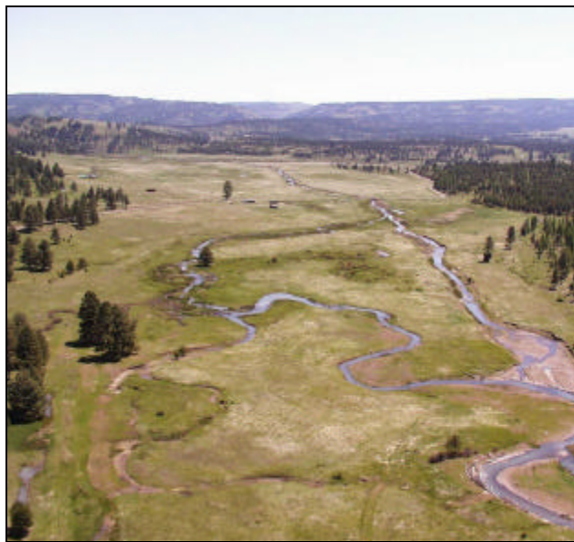
The above photo provides a downstream view of the McCoy Meadows Meadow Restoration phase I project area. Note channelized reach on right side of photo and reconnected meander channel on left. The center-left portion of the photo shows the confluence of McCoy Creek with McIntyre Creek. In July 2000, the channelized stream segments will be rehabilitated by filling portions of the channel and recontouring streambanks to develop ponds and wetland areas.
