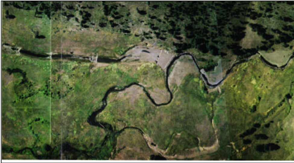
June 1998 Aerial view of Phase I project implementation. McCoy Creek was partially diverted in 1997. Rock structures installed at diversion point (center-upper of photo) was set at grade to split about 300 cfs down the new channel. The channelized reach is temporarily functioning as an overflow channel to provide recovery time in the restored channel segments. This aerial photo of upper McCoy Meadows, taken in June, 1998 illustrates restored meander channel and channelized section.
