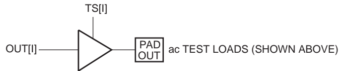
Figure 74. ac Test Loads
