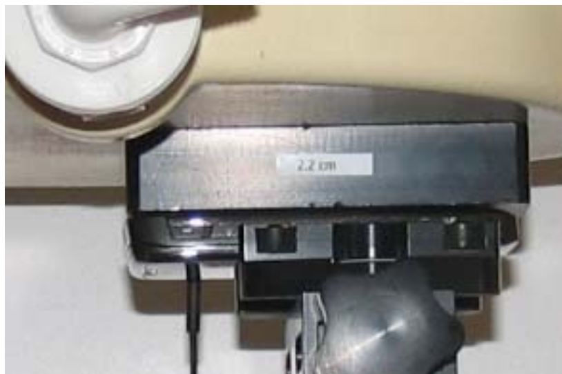
Photo of the device positioned for Body SAR measurement. The spacer was removed for the tests.
