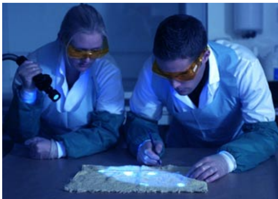
Two SKL experts searching for biological traces suitable for DNA analysis. Traces of sperm and other bodily secretions fluoresce when illuminated with light of certain wavelengths.
