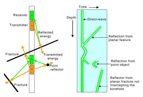
**Figure 2.** Transmitter and receiver antenna arrangement for borehole-radar reflection logging and the typical reflection patterns from planar and point reflectors.
