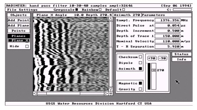
**Figure 4.** Screen capture showing the use of RADINTER software to interactively interpret borehole-radar reflection logs.
