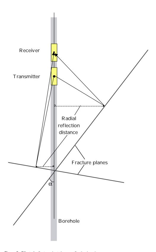
Figure 5. Effect of reflector orientation on reflection imaging.
