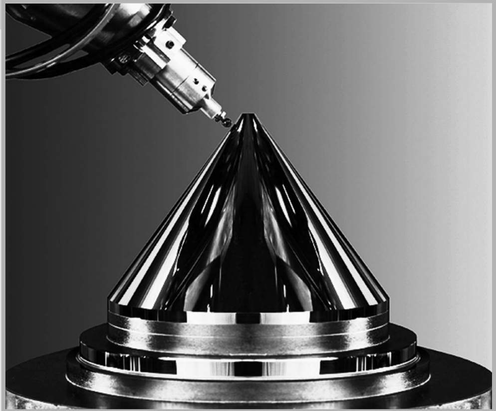
Pictured here is the large optics diamond turning machine and an aspherical mirror that the machine was first able to produce.
