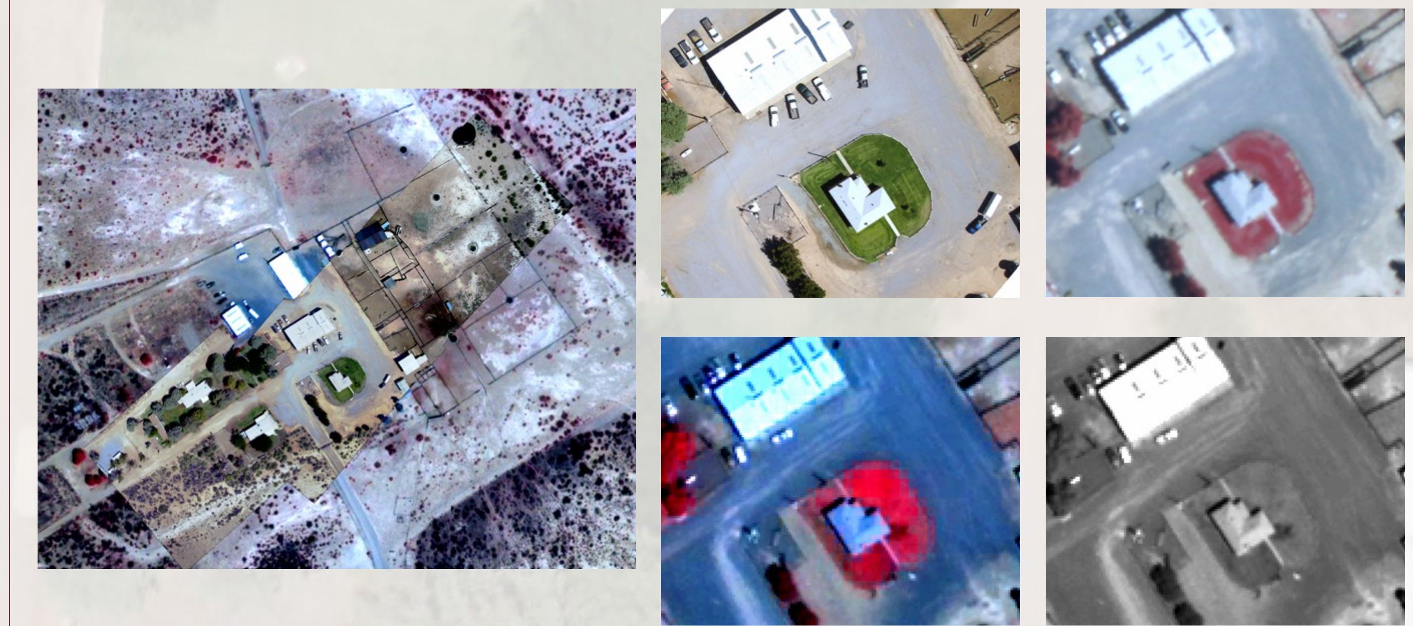
Mosaic of orthorectified MMA images overlaid on panchromatic QuickBird satellite image (left). Comparison of MMA image at 5 cm resolution (top middle), aerial photo at 24 cm resolution (top right), panchromatic band of QuickBird image at 61 cm resolution (bottom right), and panchromatic band of QuickBird image at 61 cm resolution (bottom middle).
