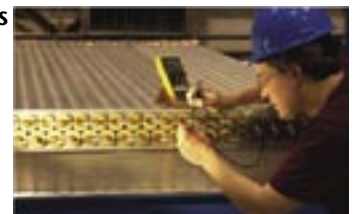
J. Andrew Green of the Physics (P) Division inspects the drift tubes that make up one pair of detectors for the muon radiography prototype.
