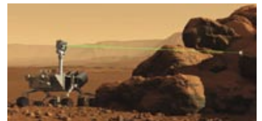
The Los Alamos laser unit, called ChemCam, uses laser-induced breakdown spectroscopy to measure the chemical content of the target samples.
