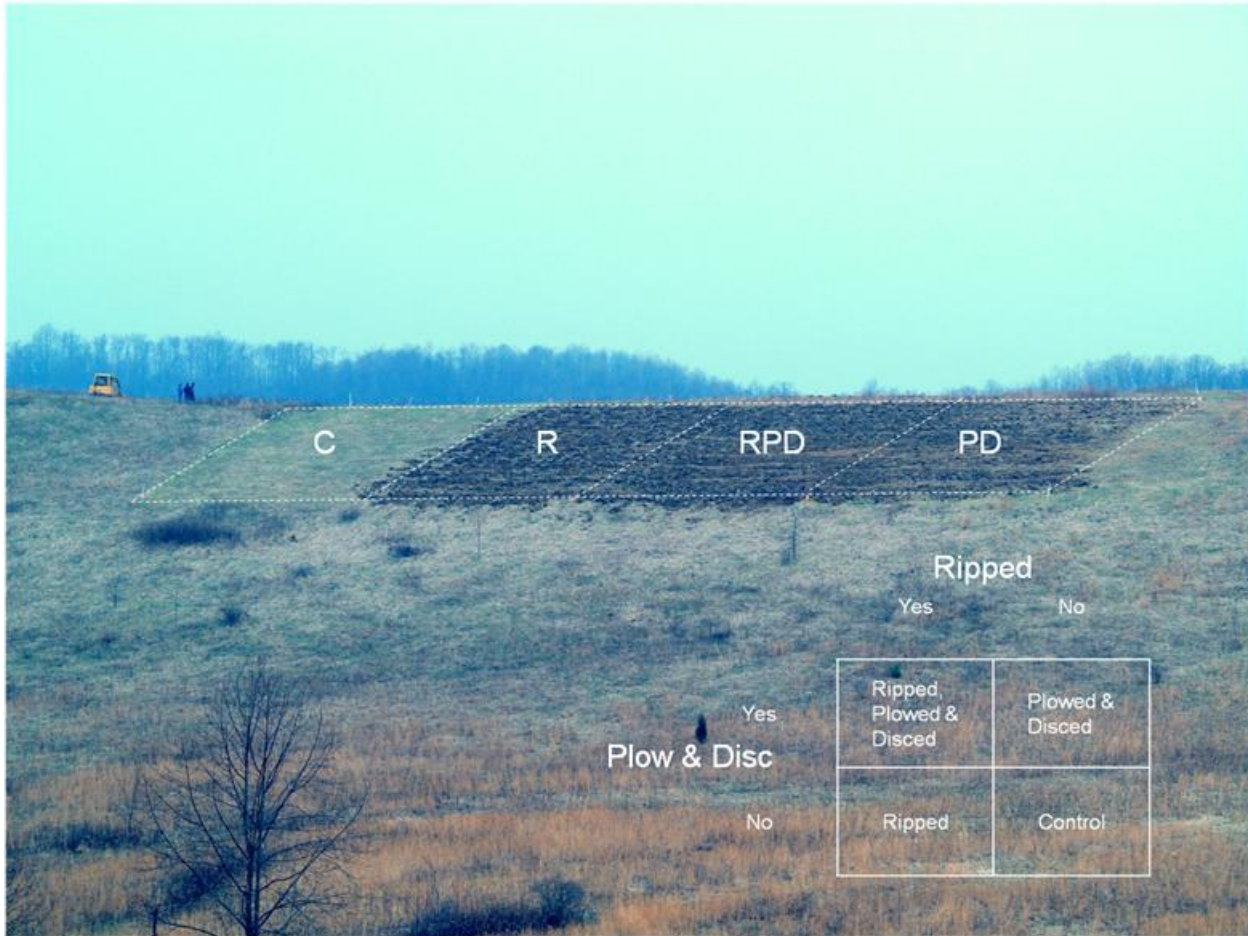
Figure 6. View of field design showing one block with control plot and three treatments: R = ripped, PD = plowed & disked, RPD = ripped, plowed & disked.
