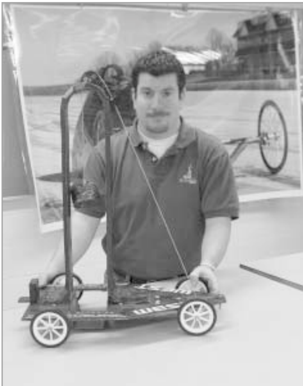
An instructor poses with the composite scrambler prototype vehicle. Its structure is 100% carbon fiber and Kevlar with a honeycomb core.
