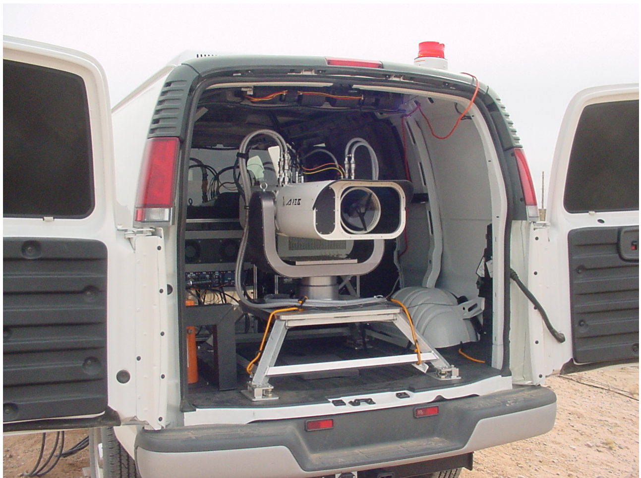
Figure 2. Photograph of the Ares UV LIF system mounted in a van ready for deployment.
