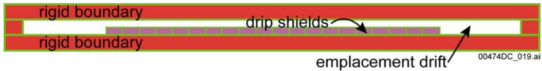
Figure 5-7. UDEC Representation of a Chain of 20 Drip Shields Linked Together at Their End Contacts
