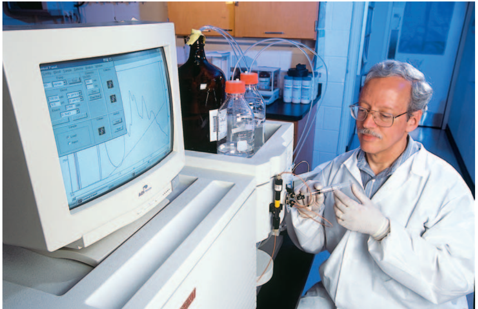
At the ARS Microbial Safety of Aquaculture Products Center of Excellence, microbiologist Gary Richards injects Vibrio extract into a chromatograph to isolate enzymes that may influence bacterial invasiveness.
