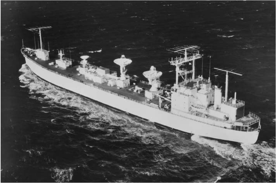
A converted Navy tanker, the Vanguard was one of the so-called “insertion ships” that tracked and communicated with the Apollo spacecraft as it performed the Trans-Lunar Injection burn, sending astronauts on their way to the Moon. (Folder 8788, NASA Historical Reference Collection, NASA History Division, NASA Headquarters, Washington DC)
