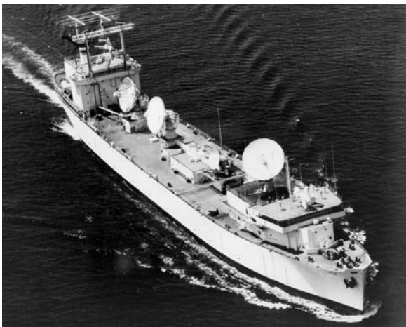
Smaller than the insertion ship, the Redstone was one of the World War II liberty ships that was converted into a reentry ship used to track and communicate with the Apollo Command Module as it reentered Earth's atmosphere towards a splash down in the Pacific. (Folder 8788, NASA Historical Reference Collection, NASA History Division, NASA Headquarters, Washington DC)
