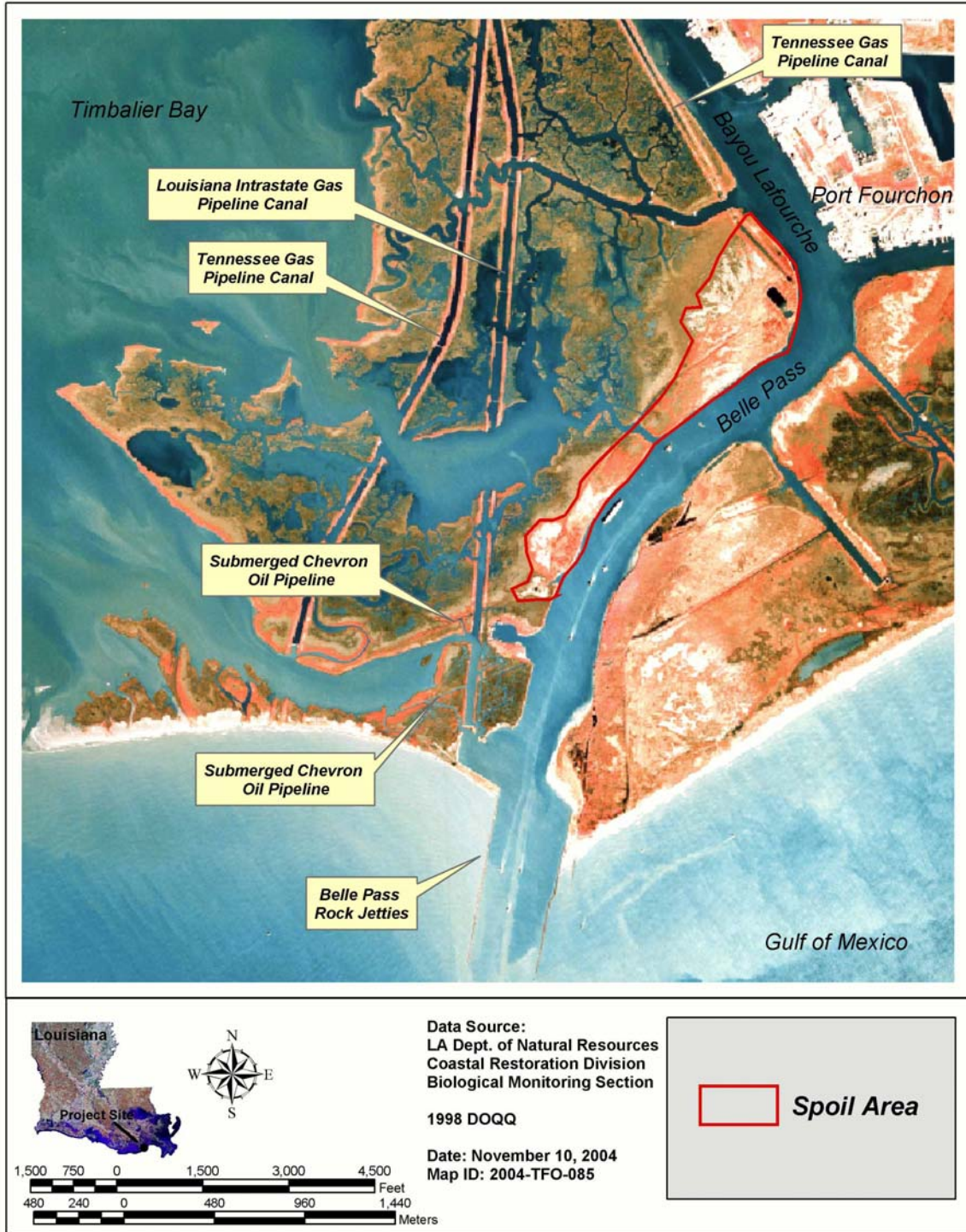
Figure 4. Anthropogenic modifications affecting hydrology and sediment distributions at the West Belle Pass Headland Restoration (TE-23) project. These alterations predate project construction.
