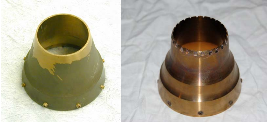
Figure 7 Convergent nozzle SMC000 (left) and modified convergent nozzle SMC021 (right).
