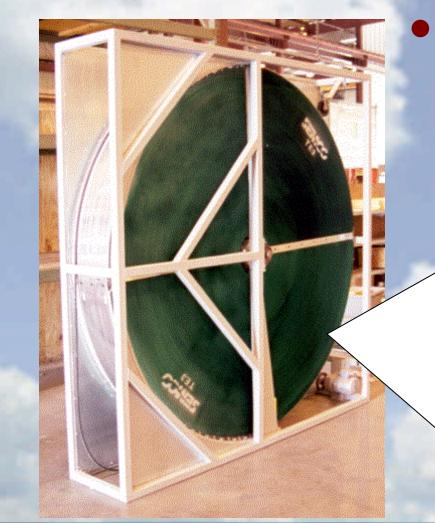
The SEMCO total energy recovers sensible (temperature) and latent (moisture) energy by up to 85%.
