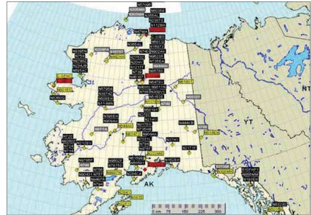
Screen capture of WebTracker image from (date). Tag colors represent status: black = parked at airport; gray = parked off airport; yellow = currently reporting; red = was reporting, but no reports within last 15-45 minutes.
