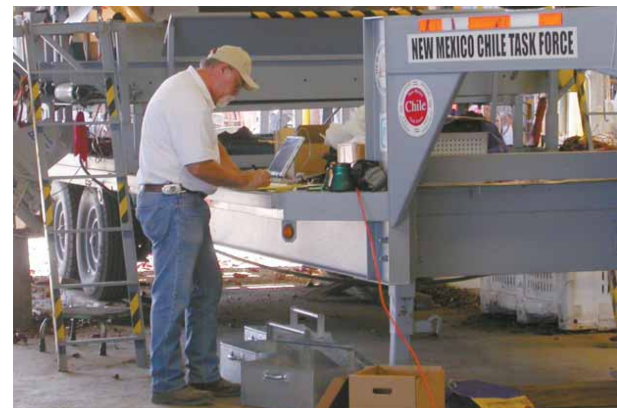
CHILE CLEANER — Ed Eaton, an agricultural engineer with New Mexico State University's Cooperative Extension Service, fine-tunes a prototype mechanical field cleaner for chile peppers. (Photo by J. Victor Espinoza)
