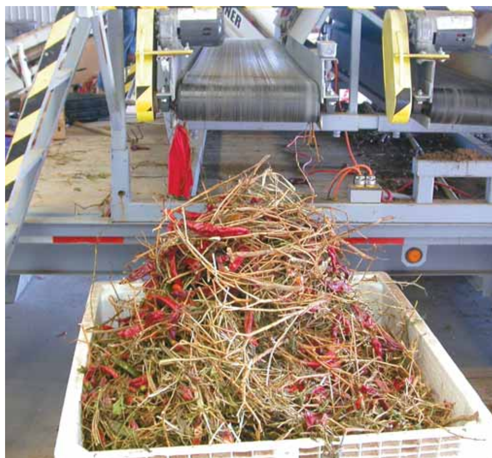
SEEING RED — A team from Sandia's Intelligent Systems Control Dept. 15234 has developed a system that uses a digital camera and software to analyze the chile and debris on a mechanical chile cleaner's conveyor belt based on color differences and provide feedback to the operator on percentages of product and waste.
