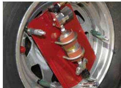
DETAIL of automatic tire pressure system, developed by Dale Petty of Petty Farm and Ranch in Clovis, N.M., with help from Sandia.
