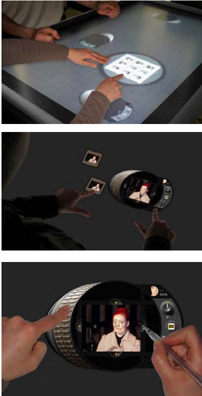
Figure 4: From the top: a user drags slides out of the shared tray; in the middle, the user positions selected pictures under the Imagetool virtual lens; at the bottom, affordances for two-hands interaction. The image can be zoomed by scrolling the left gear; and cropped by dragging the semi-opaque ledgers within the lens, which resemble the blades of a four bladed photographic easel.
