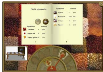
Figure 3: The Living Cookbook interface: the dial embodies the cookbook selection; video control is operated on an egg-shaped widget (second from top); portions can be specified by dragging plates on a table (bottom).
