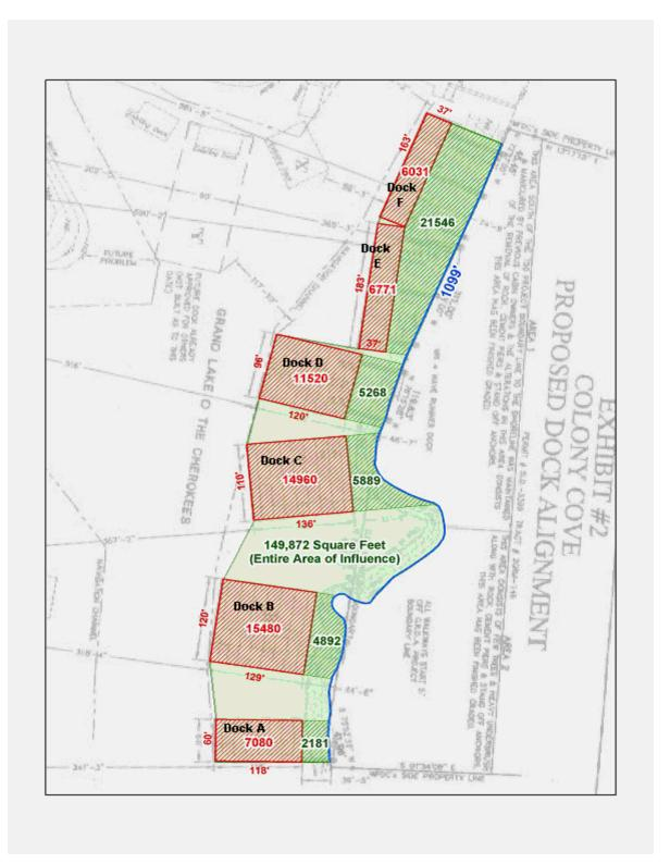
Figure 1. Layout of proposed docks at Colony Cove. Pensacola Project. FERC No. 1494-244, Oklahoma (source: Grand River Dam Authority, Application for Non-Project Use of Project Lands and Waters, filed March 28, 2003, as modified by staff.)
