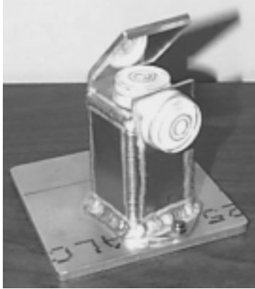
Figure 1: Prototype Quasi-steady Acceleration Direction Indicator for drop tower tests.
