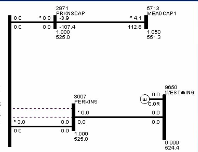
BUS # 2970 PRKNSPST525.0 TYPE 1 AREA 14 ARIZONA ZONE 158 SRP TSW VOLTAGE 1.00000PU 525.000KV ANGLE 0.00Deg
