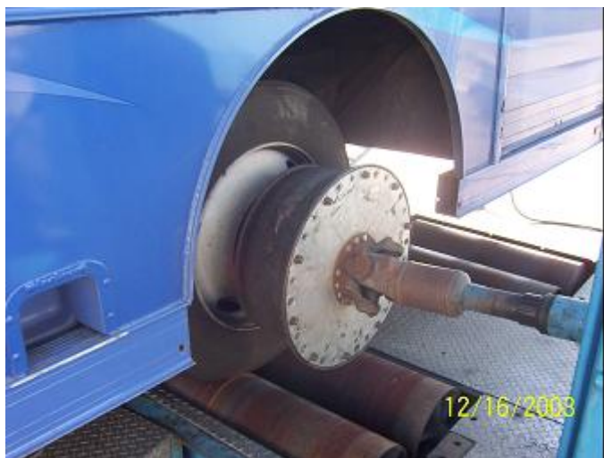
Figure 9. Close-up photo of hub adapters coupled to drive axle.
