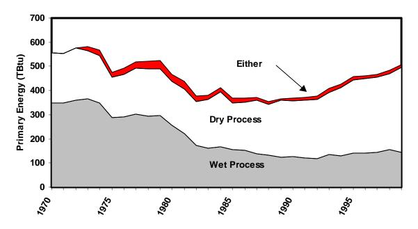
Figure 4. Primary Energy Consumption in U.S. Cement Production by Process, 1970 to 1999 (expressed in TBtu). Source: derived from USGS, various years.
