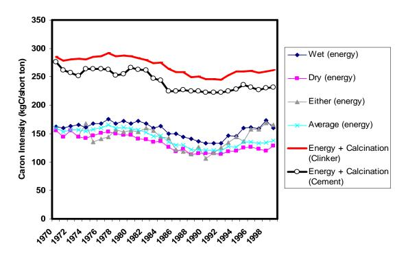
Figure 8. Carbon Intensity of U.S. Cement and Clinker Production, 1970 to 1999 (expressed in kgC/short ton of product). This graph excludes use of wastes as kiln fuel between 1977 and 1992, as USGS did not collect this data before 1993. See below for a discussion on the impact of including assumptions on waste use. Source: derived from USGS, various years.
