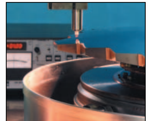
Machining metal up to 1.65 meters in diameter and at a precision of 2 micrometers is possible with LODTM.
