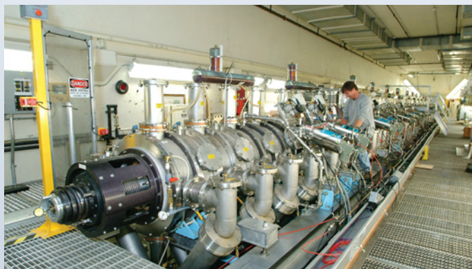
Mechanical technologist Keith Lewis works on the Flash X Ray (FXR) accelerator, an important diagnostic tool for hydrodynamic testing. The firing chamber is behind the wall at the far end of FXR.
