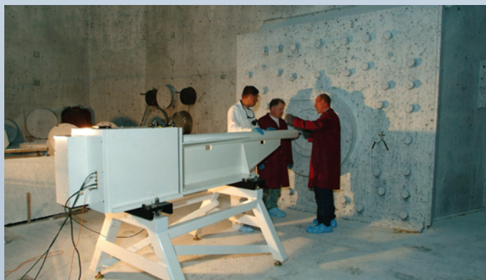
John Given, Steve Bosson, and Jack Lowry adjust the quality of the FXR beam, which enters the firing chamber through the port behind them. FXR is on the other side of the wall to protect it from explosive debris.
