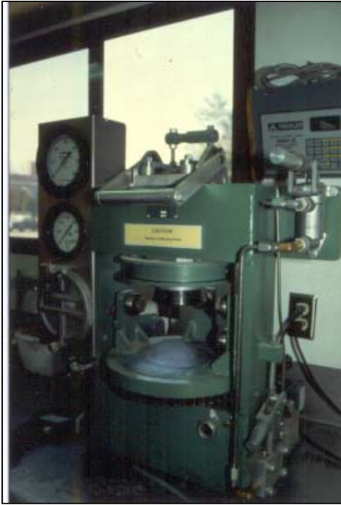
Figure 5. 1987, Rainhart Company, Gyratory Shear Test Machine
