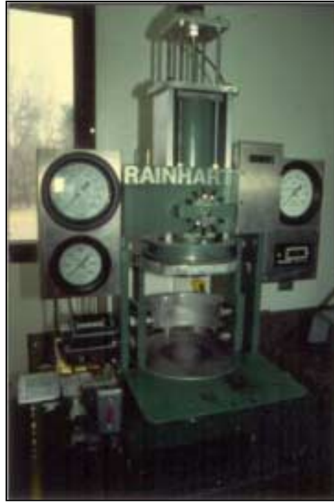
Figure 6. 1991, Rainhart Company, Modified Gyratory Shear Test Machine
