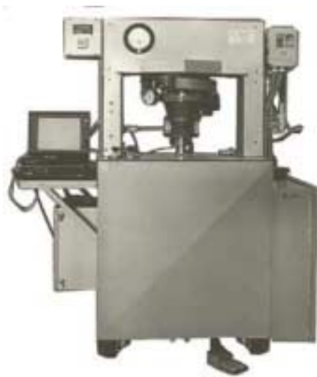
Figure 2. U.S. Corps of Engineers Gyrotory Kneading Compactor
