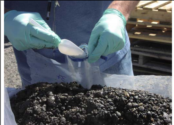
Figure 3. A grab sample of Hanford formation aquifer sediments being sampled for microbiologic characterization. Aseptic sampling methods will be used for the deep characterization borehole, 2-25.
