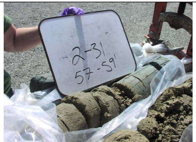
Figure 4. Transition between oxic and anoxic zones in fine-grained sediments of the upper Ringold Formation. The anoxic zone with distinct greenish blue coloration is located approximately 0.3m below the Hanford-Ringold contact. This oxic-anoxic interface has been intersected by all boreholes drilled to date in the IFC well field.
